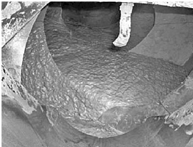
FIGURE 24.7 Creamy texture appearance of fresh ECC in mixing drum of a ready-mix truck. (From Lepech, M.D. and Li, V.C., ACI Mater. J. , 2008.)
